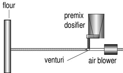
Pneumatic conveying of flour fortificants from the feeder to the flour collection conveyor has one key advantage. It permits the feeder to be located anywhere in the mill, allowing it to be conveniently located or added to a mill retroactively. However a pneumatic conveying system requires the investment of additional equipment such as blower, valve and piping.
