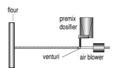
Pneumatic conveying of flour fortificants from the feeder to the flour collection conveyor has one key advantage. It permits the feeder to be located anywhere in the mill, allowing it to be conveniently located or added to a mill retroactively. However a pneumatic conveying system requires the investment of additional equipment such as blower, valve and piping.
